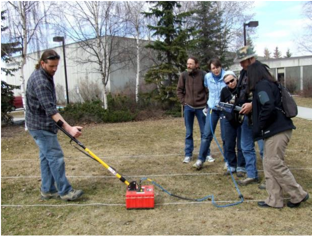
Figure 2: Ground penetrating radar measuring soil composition. " Ground Penetrating Radar " by Travis S. is licensed under CC BY-NC 2.0 .
