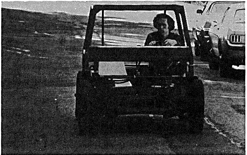
Fig. 5-3. Testbed Electric Vehicle for Full Scale Dynamic Tests of the Power Coupling Between the Roadway Power Source and an Electric Vehicle.
