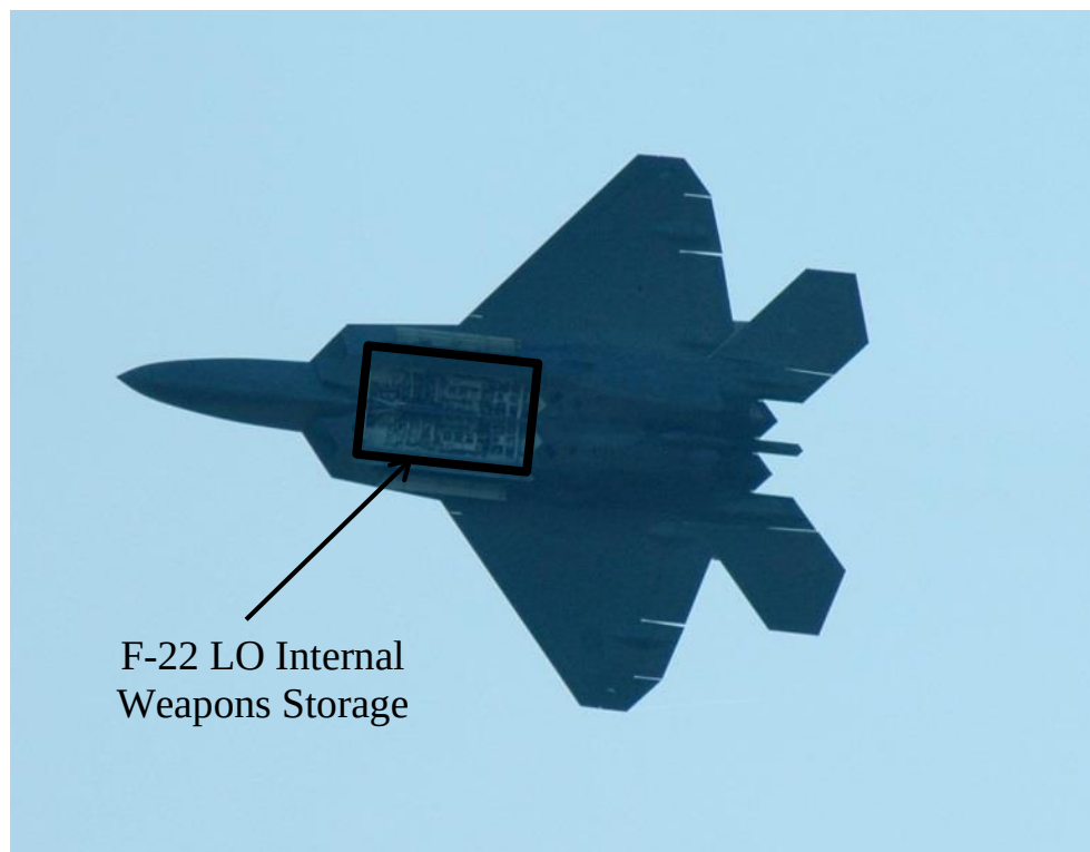
Figure 6.1-8. F-22 internal weapons storage volume.
