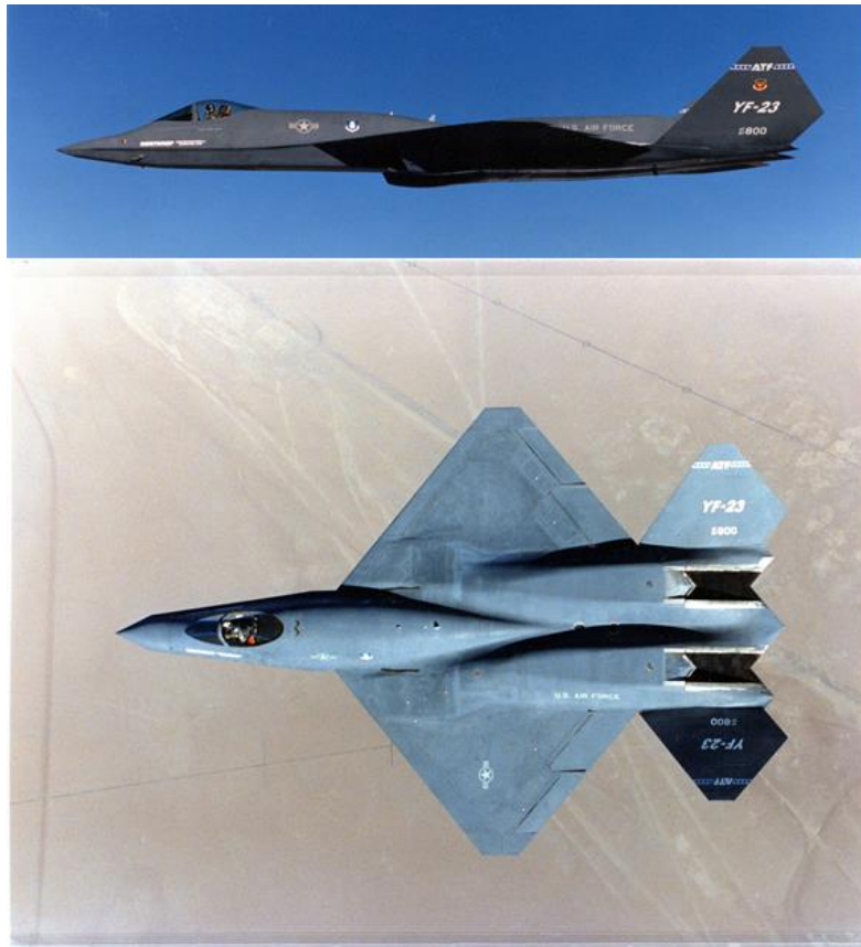
Figure 6.4-1. Northrop YF-23 side view and top view showing trapezoidal planform and area ruling features.
