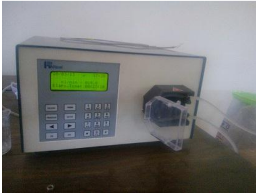
Figure 3.5 Peristaltic Pump used as a part of the experimental set up showing readings monitor and the water carrying pipe.
