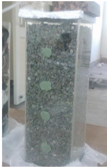
Figure 3.22 Gravel reactor of column height 30cm used in the experiments
