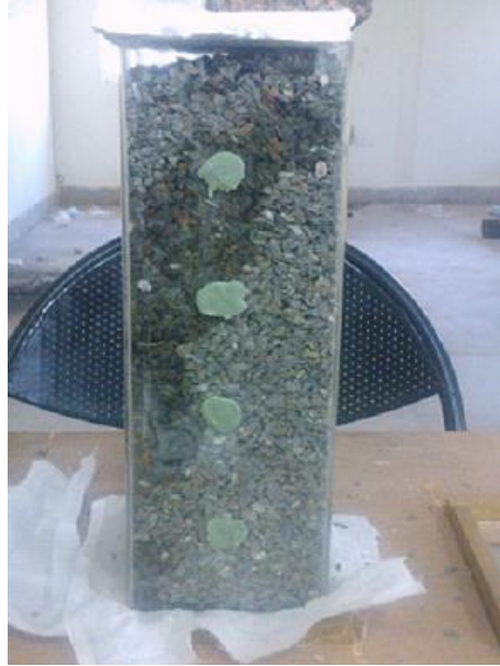
Figure 3.4 Thirty centimetre acrylic column filled with gravels
