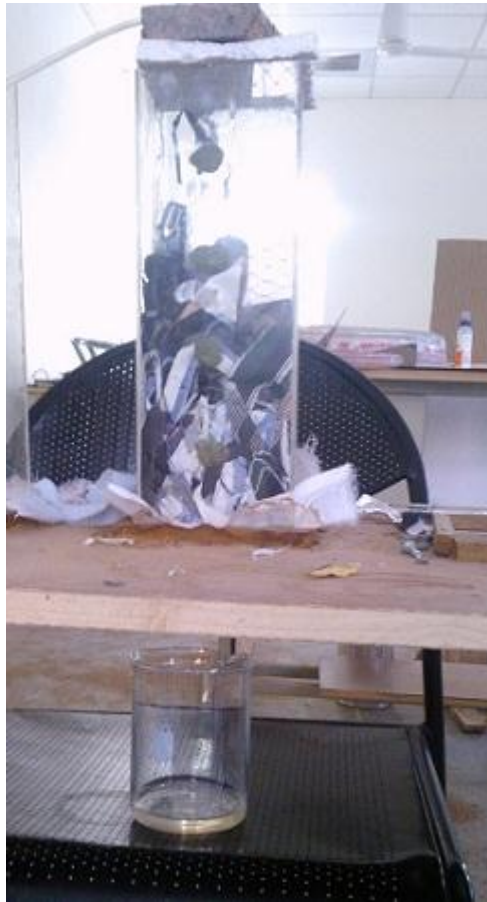
Figure 3.23 Discharged effluent was collected in a beaker and noted consecutively for calculation of cumulative time as well as for flow rate of effluent
