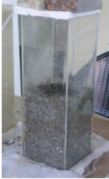
Figure 3.21 Gravel reactor of height 15cm used in this study
