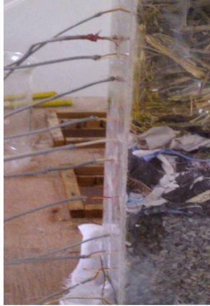
Figure 3.8 Thermocouples inserted in the reactor
