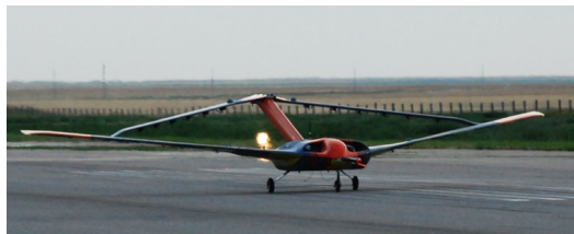
Figure 1.10: Stiff SensorCraft geometrically scaled to 1/9^{\text{th}} of a Boeing/AFRL concept [4].
