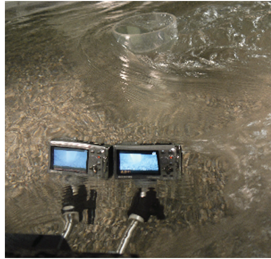
Figure 6. The cameras recording the scour hole, mounted on the sidewalls of the flume. Flow direction is from left to right.
