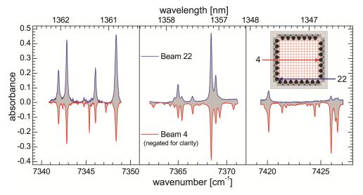
Fig. 4. Absorption spectra measured during a single scan of the TDM 3-FDML laser operating at 50.24337 kHz ( $\sim$ 20 microseconds). Each panel shows the spectra measured by one of the three FDML lasers.
