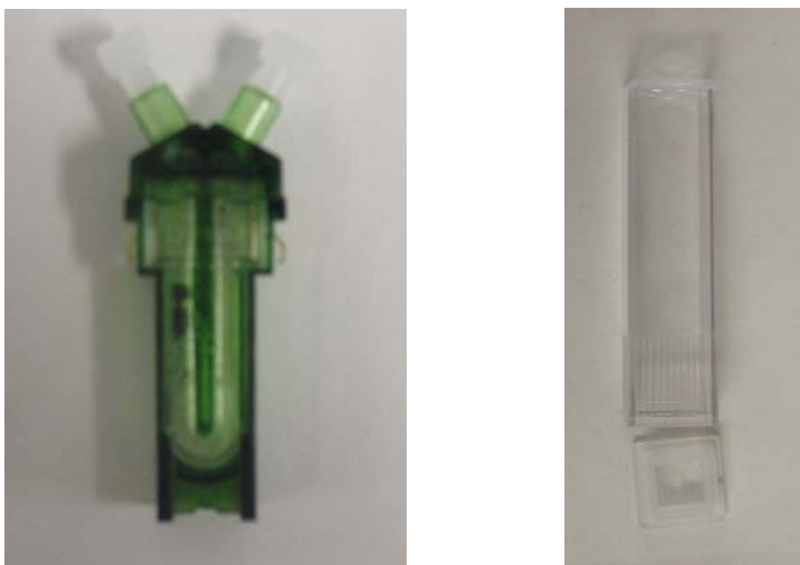
Figure 38: Digital picture of cuvettes used for the zeta potential (left) and particle size (right) measurements
