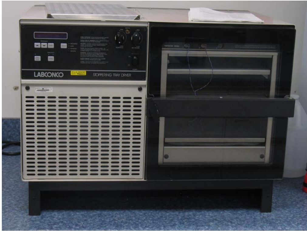
Figure 41: Digital picture of the Labconco Freezone Stoppering Tray Dryer
