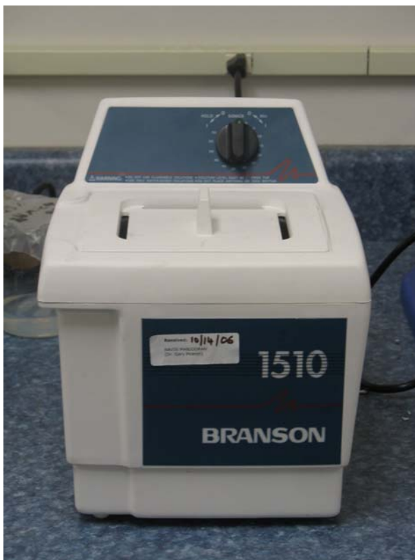
Figure 35: Digital picture of Bransonic 1510 ultrasonic bath
