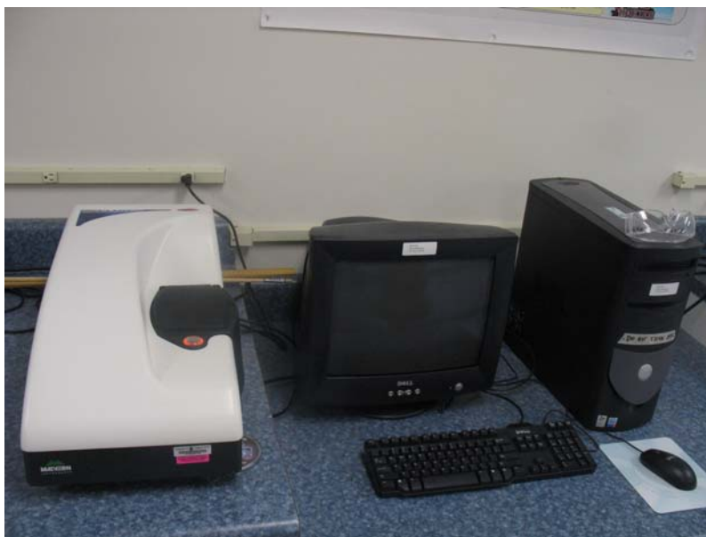
Figure 37: Digital picture of the Malvern nano zetasizer ZS
