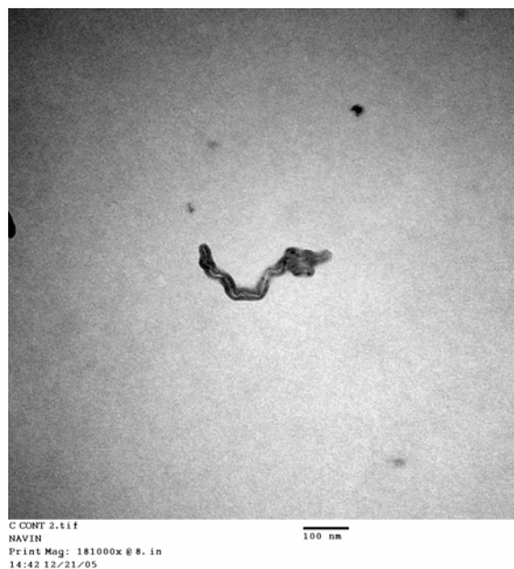
Figure 186: TEM image of carbon nanotubes
