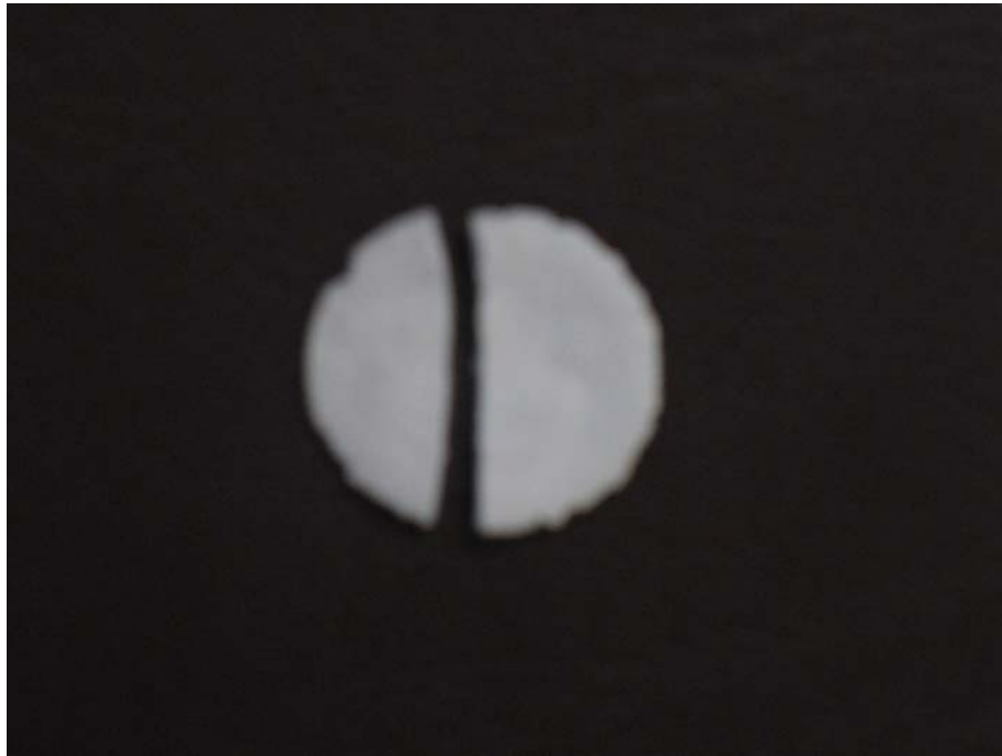
Figure 163: Digital picture showing the sample failure along the diameter during the diametric compression test
