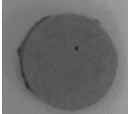
Figure 141: Digital image of the \alpha -SiC/H 2 O/ \alpha -SiC based freeze cast sample at 25 °C
