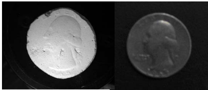
Figure 140: Digital image of the \alpha -SiC/H 2 O/LGG based freeze cast sample at 25 °C (left) and a quarter (right)
