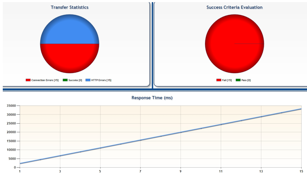
Figure A.3: Having blocking calls to the LumenHaus controller would give the perception that the web services are down if the controller failed.
