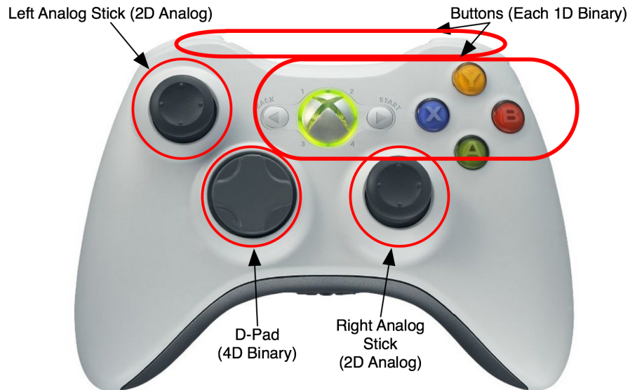
Figure 5.2: The XBox controller breakdown into primitive devices, each with a number of dimensions, nature and value range. ( Courtesy of Microsoft Hardware www.microsoft.com/hardware 2010) Public Domain
