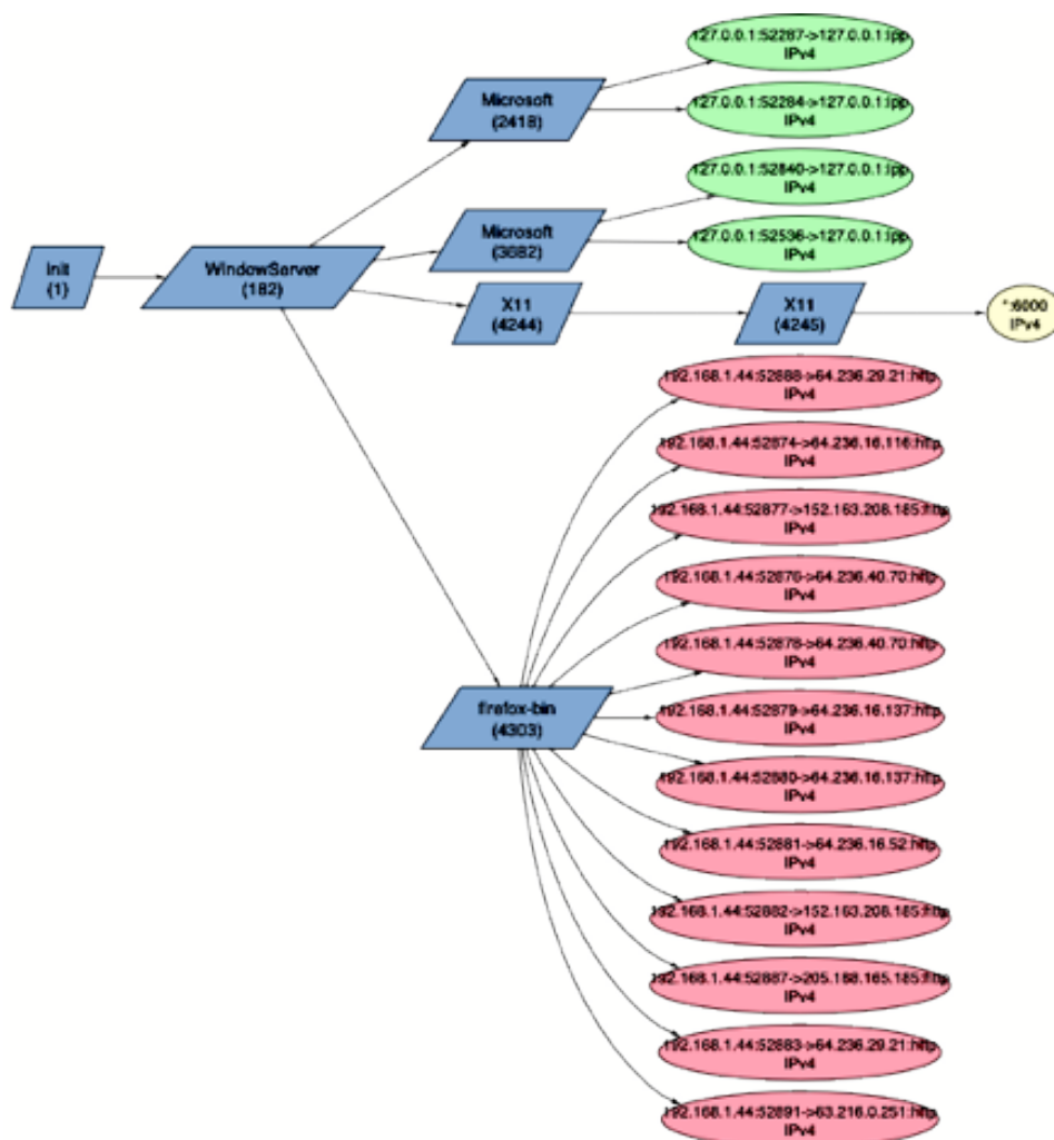
Figure 31: Screenshot of psgraph output showing that application Firefox has several open connections.
