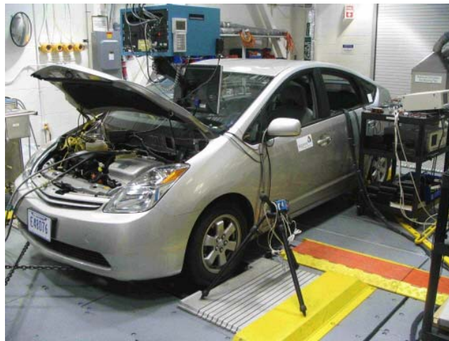
Figure 5.1 Test vehicle, 2004 Toyota Prius, on a dynamometer in ANL
