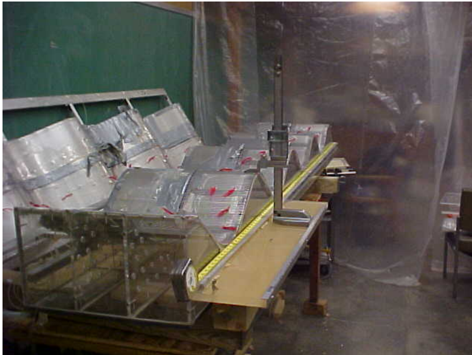
Figure A.2: Side Wall Geometry Measurement Setup
