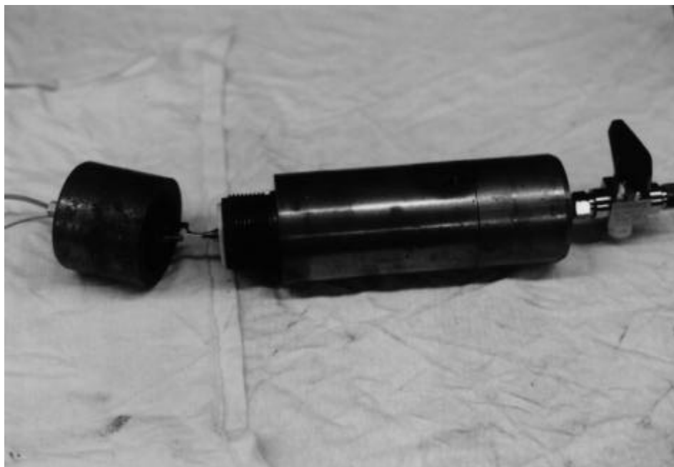
Plate 4-2: Inserting Test Charge into Test Vessel, Note Seal is in Place on Bomb.
