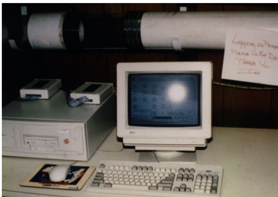
Plate 3-10: Automatic Data Logging System.
