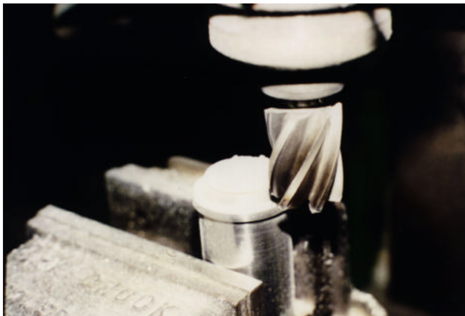
Plate 3-6: High-Speed Cutter Facing Top of Sample.
