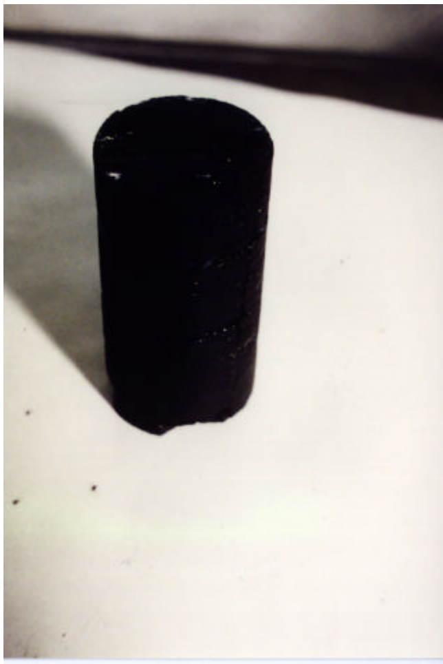
Plate 3-3: Sample after Diameter Reduction, Faceplate Removed.
