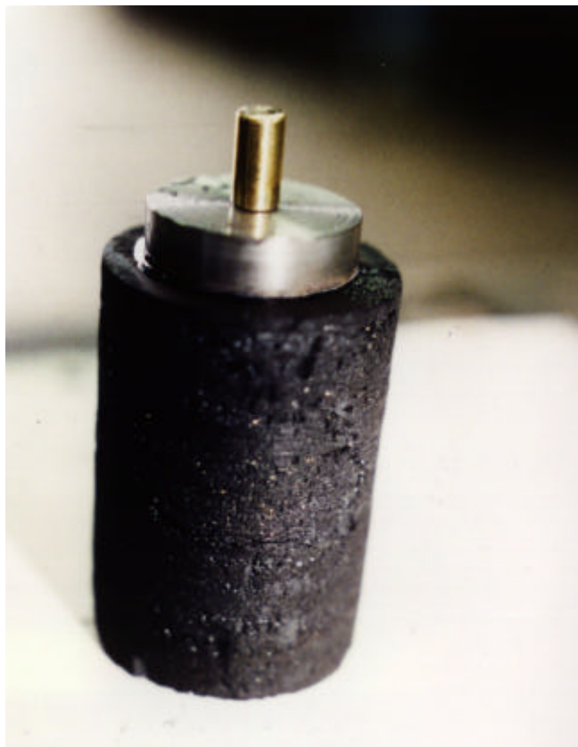
Plate 3-1: Sample Ready to be Placed into Lathe, with Faceplate Attached.
