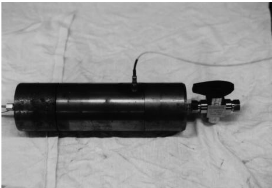
Plate 4-5: Pressure Transducer Connected to Power Supply Lead.
