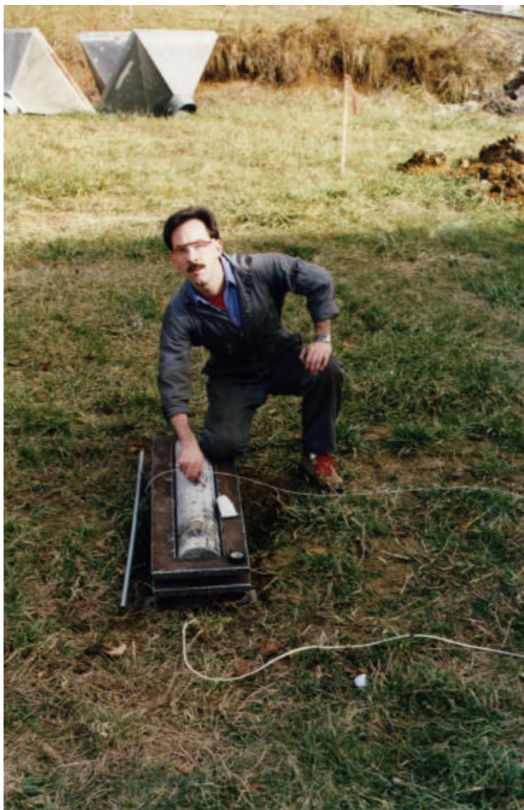
Plate 6-4: Installing Pressure Transducer into Large-scale Bomb.
