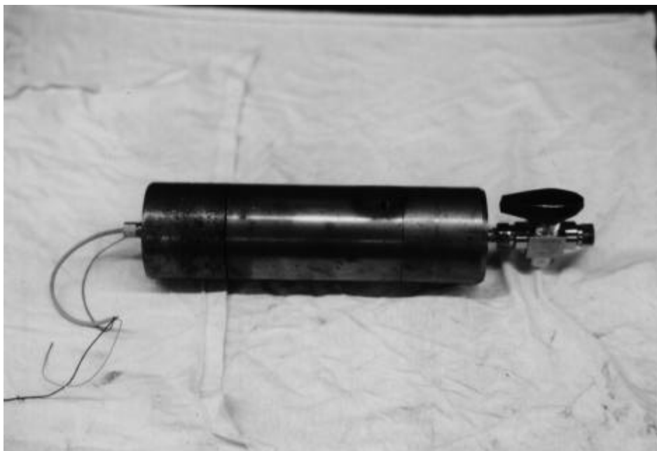
Plate 4-3: Test Vessel Closed, Valve Open, Transducer not In-place.
