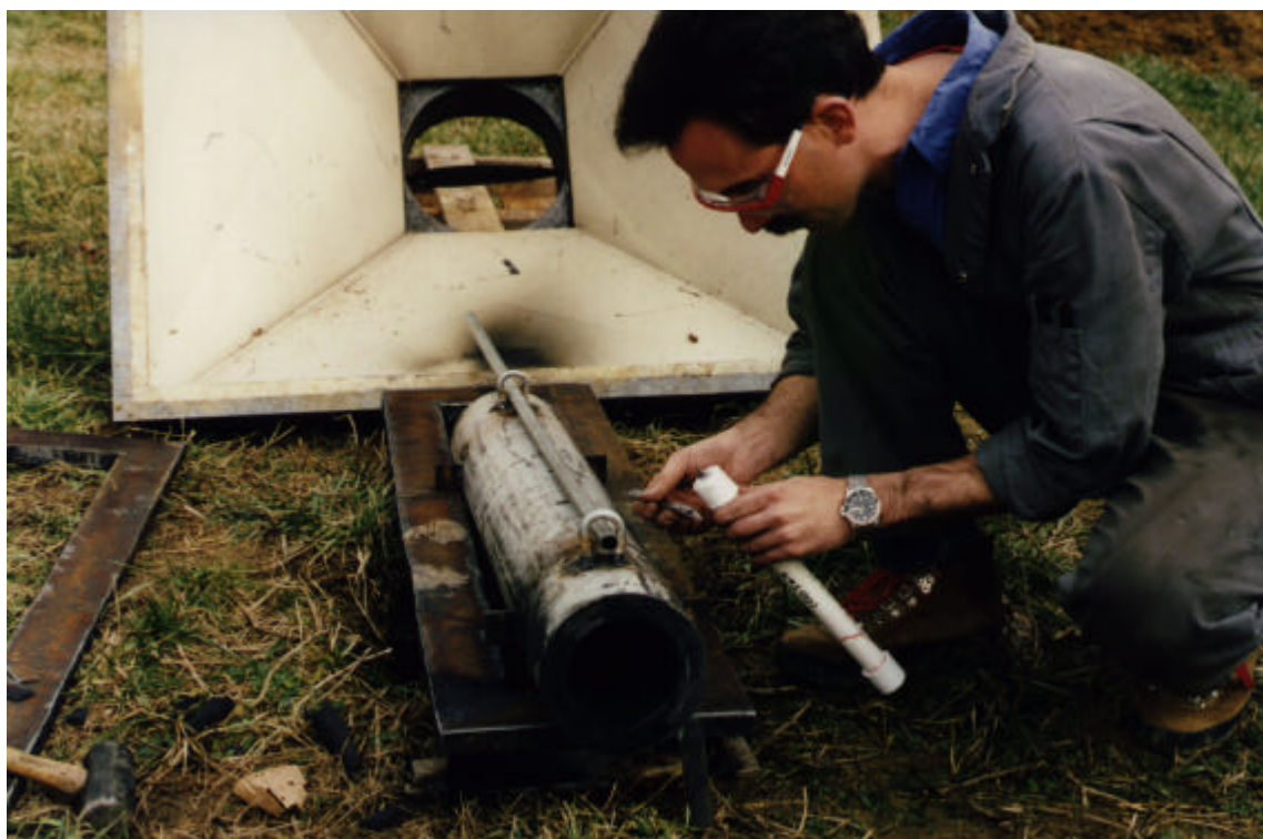
Plate 6-2: Preparing to Arm Propellant Charge with Igniter Charge.
