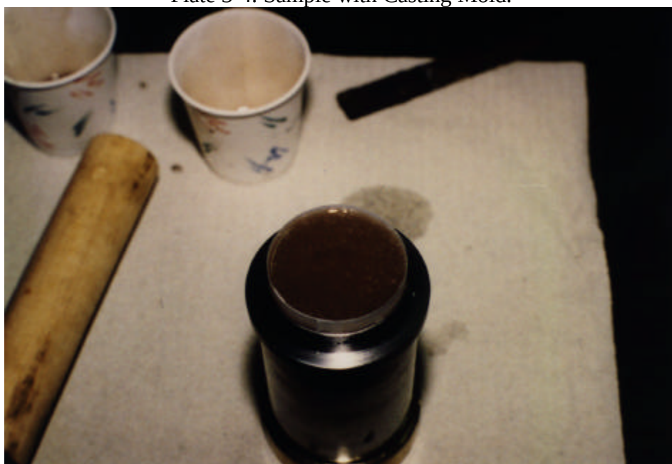
Plate 3-5: Mold with Resin Top Cap Poured.
