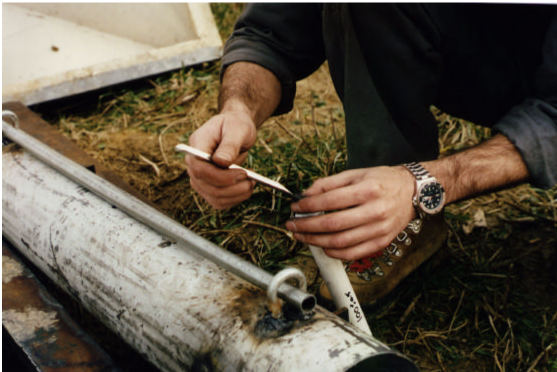
Plate 6-3: Loading Ignition Charge into Igniter Tube.
