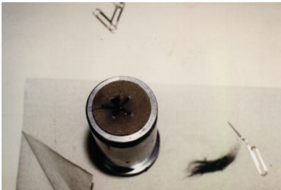
Plate 3-9: Steel Wool in Lower Vent Holes, Mold Base Cap Removed.
