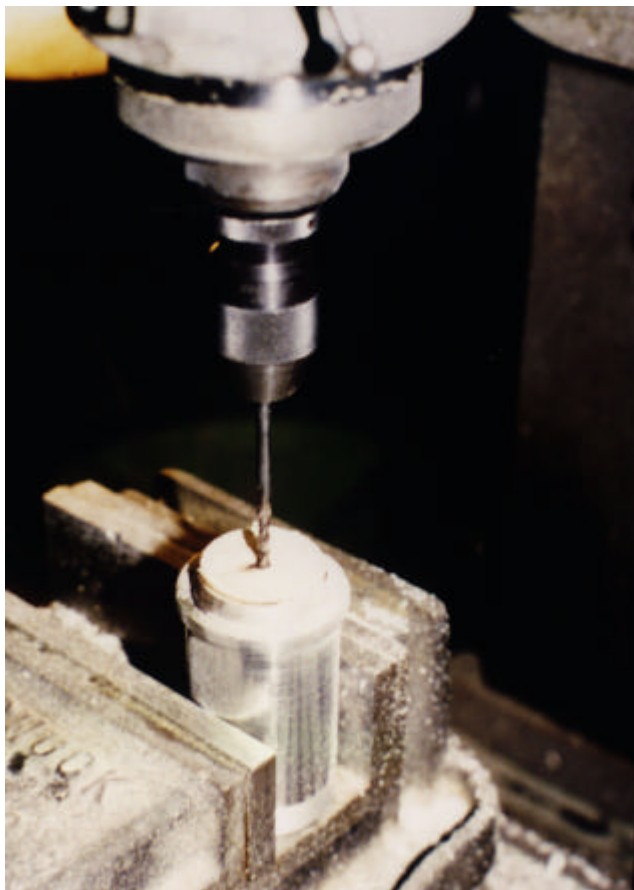
Plate 3-7: Drilling Center Hole Into Sample.
