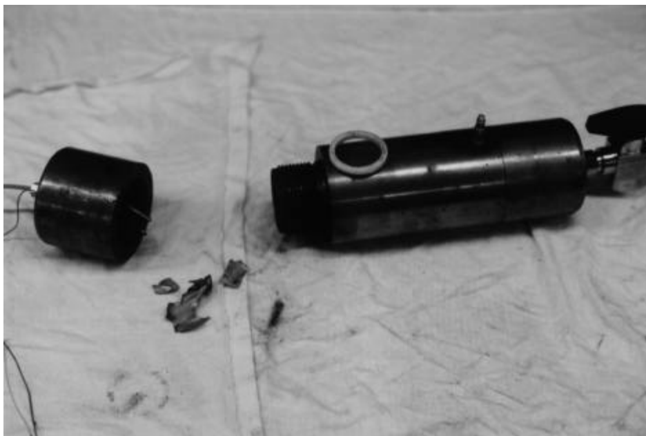
Plate 4-7: Debris Removed from Test Shot.
