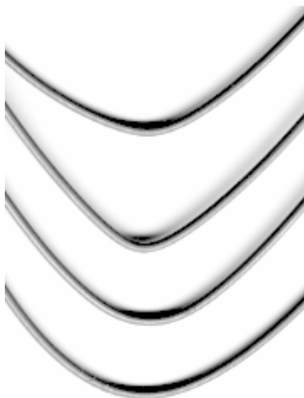
Figure 2.2: Examples of the bends of various wireform springs produced by hand forming the bend.
