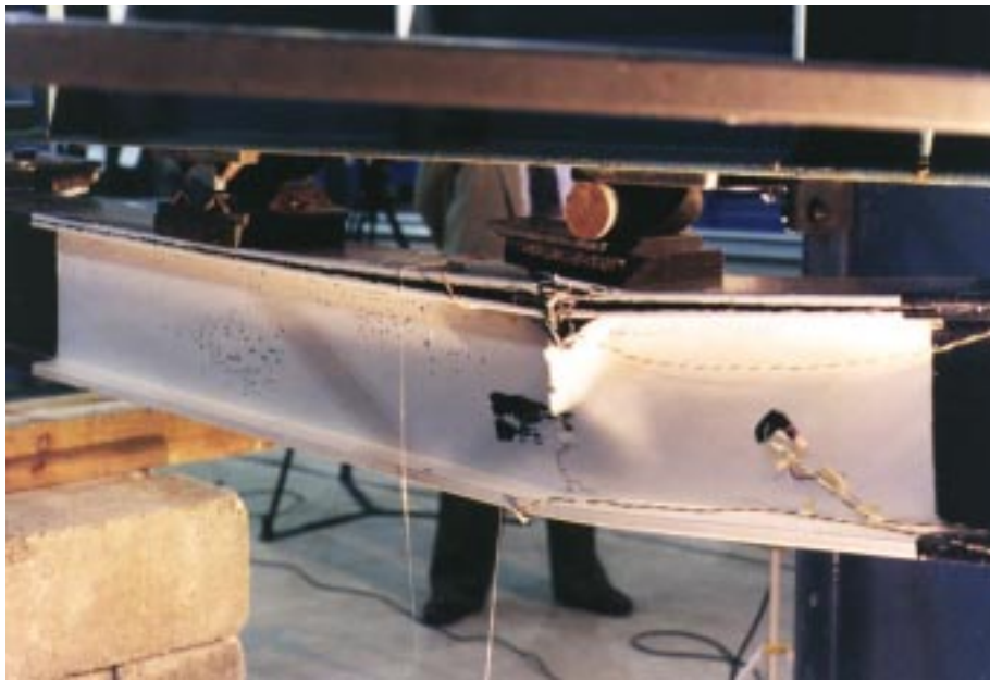
Figure 3-5. Failure of vinyl ester beam under four-point bending.
