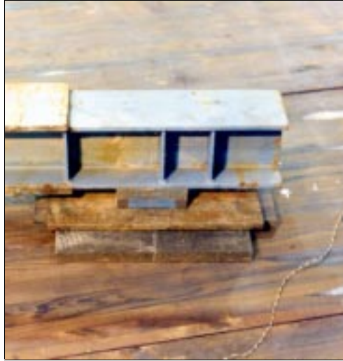
Figure 2-12. Close-up of wheel patch underneath spreader beam.
