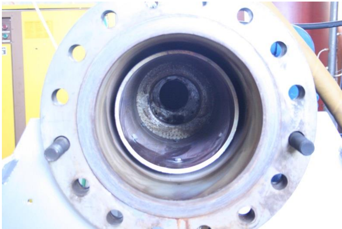
Figure D-5. Finished combustor liner as installed in the VT Aerothermal Rig
