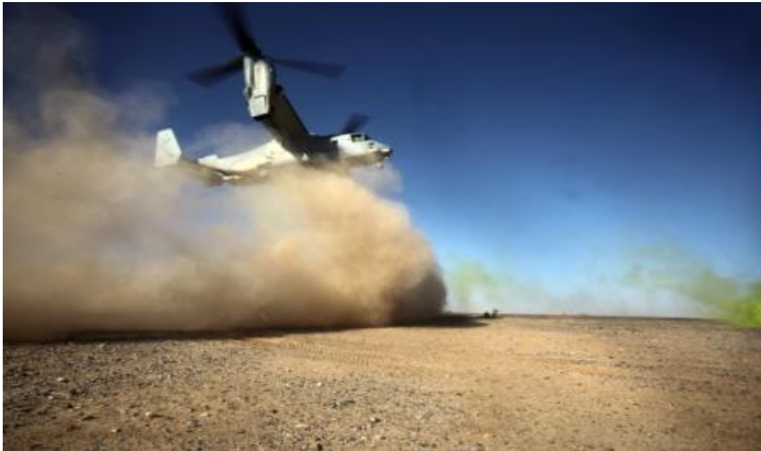
Figure 4-1. Example of sand ingestion in desert conditions
