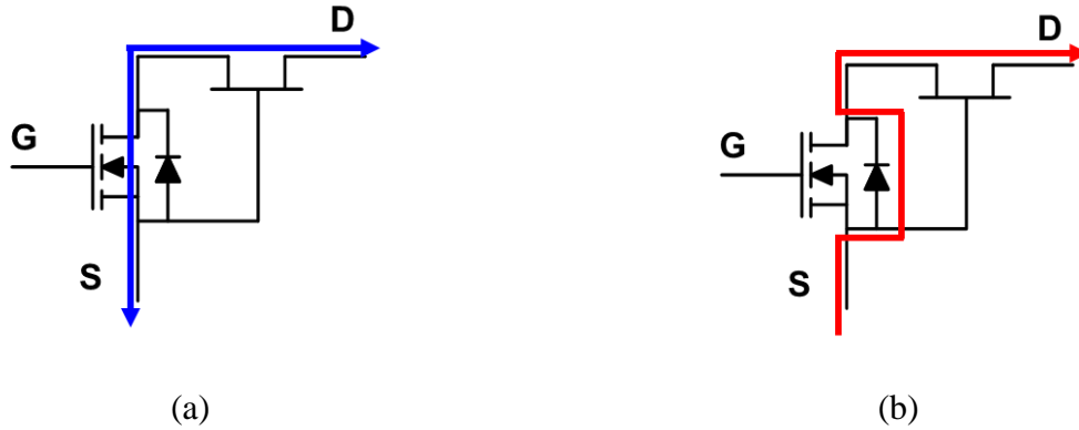
Figure 1.10 Conduction principle of cascode GaN HEMT, (a) V_{gs}=10V , (b) V_{gs}=0V
