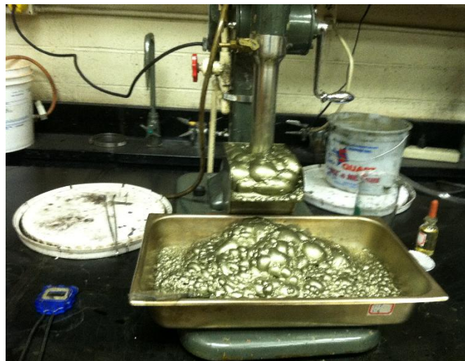
Figure 2-4: Chalcopyrite flotation using Lab scale Denver flotation cell
