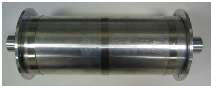
Figure 7.8: Silencer with 13 inch long expansion chamber with RVC foam lining and an airflow channel with bends (Sesler, 2003) [fair use].
