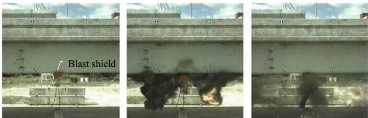
Figure 5-5: Bottom flange simulated fracture by explosion in Test 1 (Barnard, et al., 2010).
