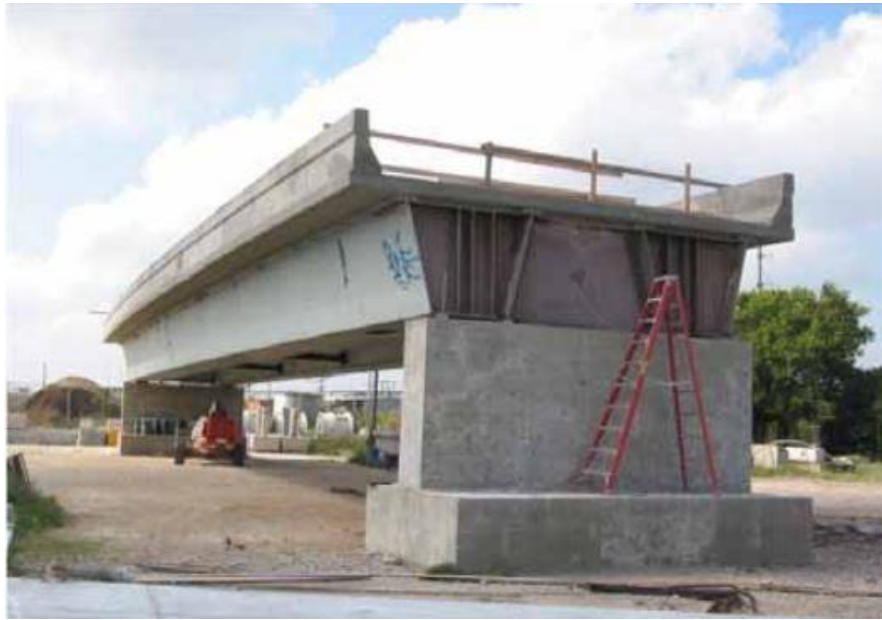
Figure 5-1: Twin box-girder test bridge (Barnard, et al., 2010).
