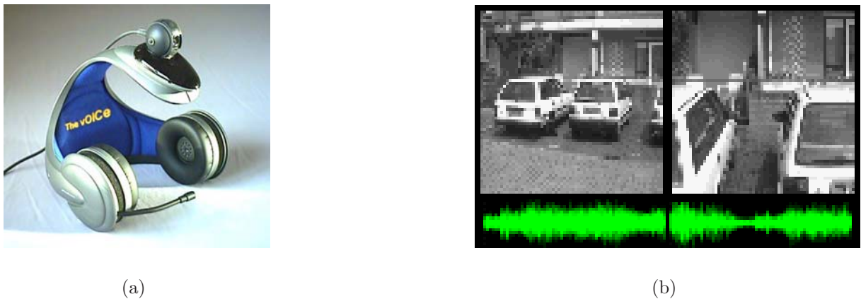
Figure 1.7: (a) The vOICe system and (b) an example of its image-to-sound rendering.
