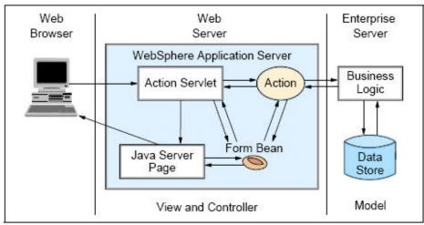
Figure 3 Struts structure
