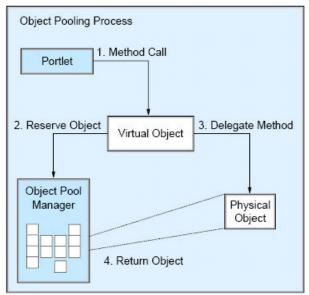
Figure 5 Object pooling process
