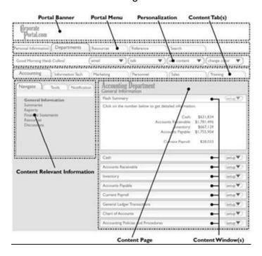
**Figure 2-2:** Main components of the web portal user interface.
