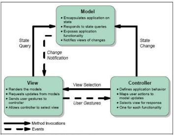
Figure 1 The Mode-View-Controller design pattern
