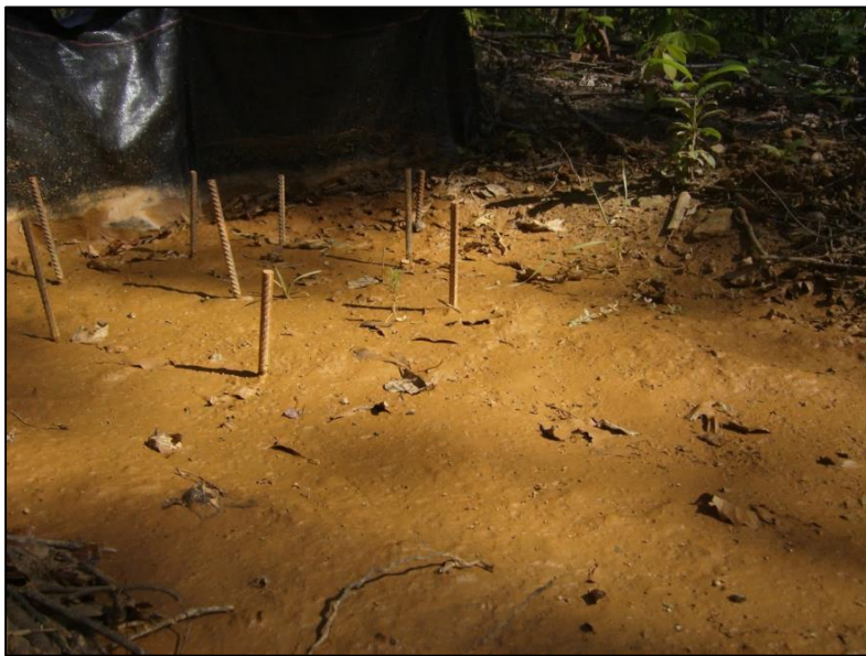
Figure 3.2. Silt fence catchment area with rebar pins marking the location of measurement.
