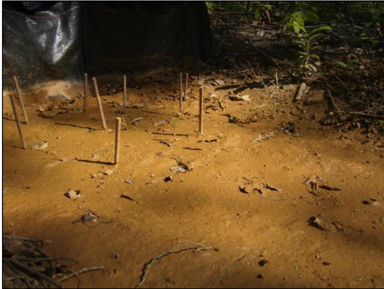
Figure 2.3. Silt fence catchment area with rebar pins marking the location of measurement.
