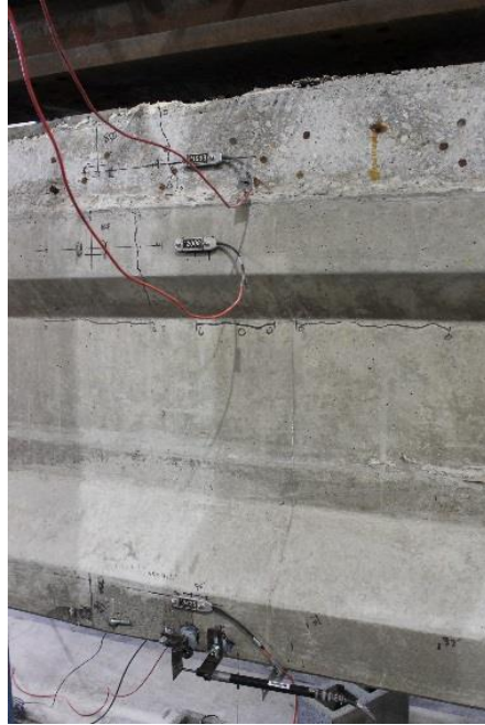
Figure 21- LVDT and Three Strain Transducers to Obtain Strain Profile
