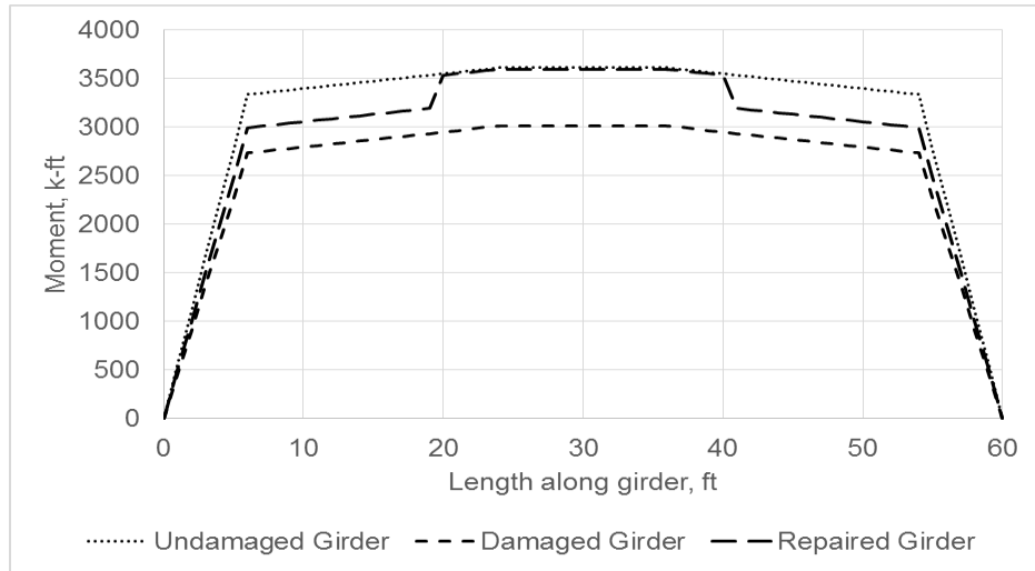
Figure 125- Moment Capacity along the Length of the Girder for the Eight Strand Damage Pattern
