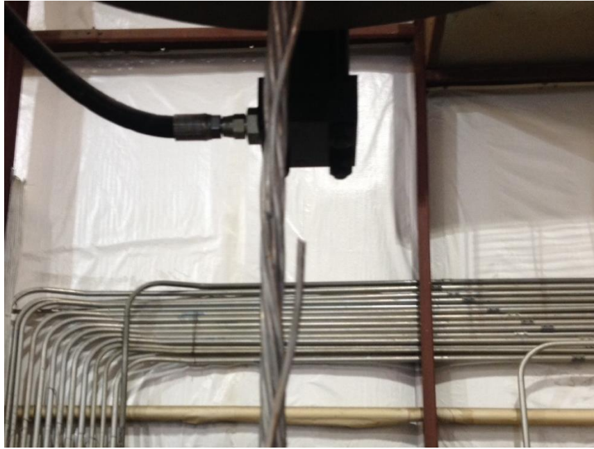
Figure 98- Prestressing Strand Rupture at Ultimate Tensile Strength
