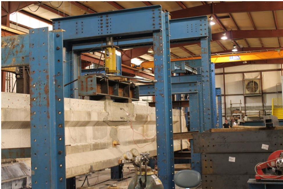
Figure 55- Test 4 Loading Set-up
