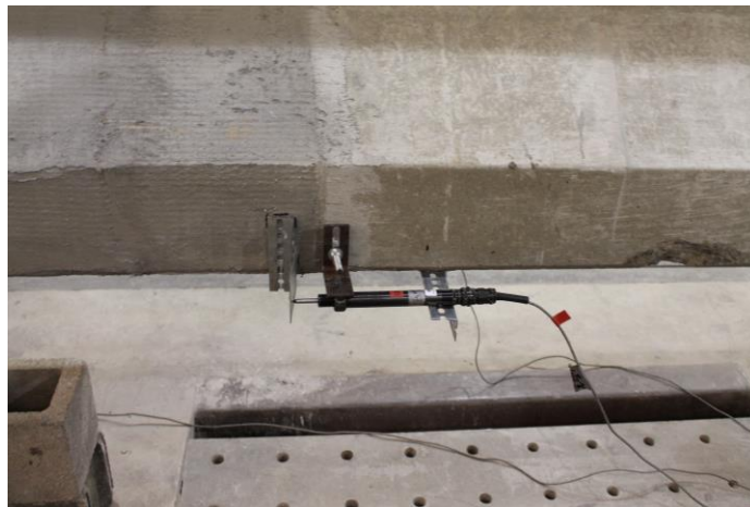
Figure 20- LVDT in place on the side of a girder
