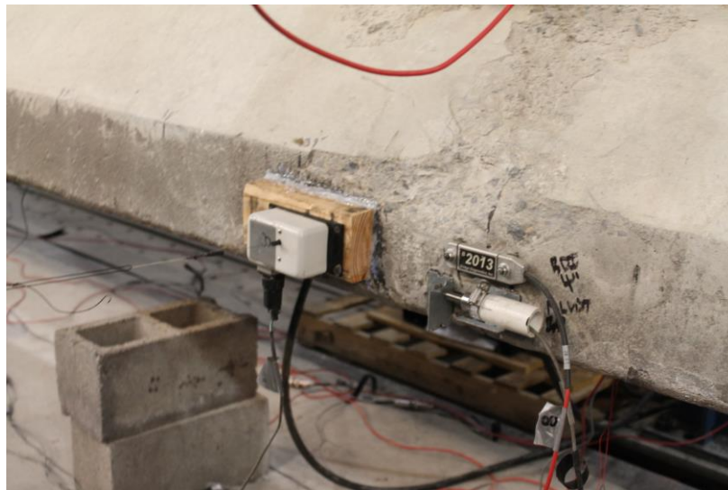
Figure 19- Potentiometer to find Lateral Displacement; MLVDT and Strain Transducer to Obtain Strain Profile
