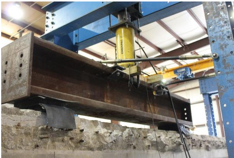
Figure 41- Test 2 Loading Set-up
