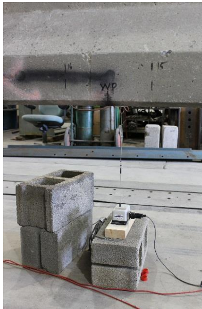
Figure 18- Potentiometer Used to Measure Downward Deflection
