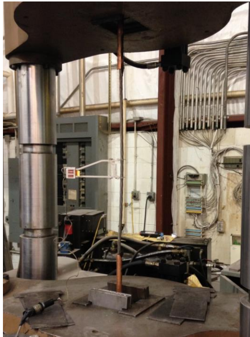
Figure 15- Tension Testing of Prestressing Strands
