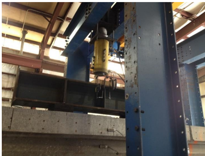
Figure 22- Test Set up with Actuator, Load Cell, Spreader Beam, and Rubber Pads
