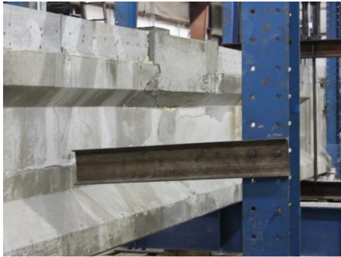
Figure 25- Bracing Frame to Prevent Tipping
