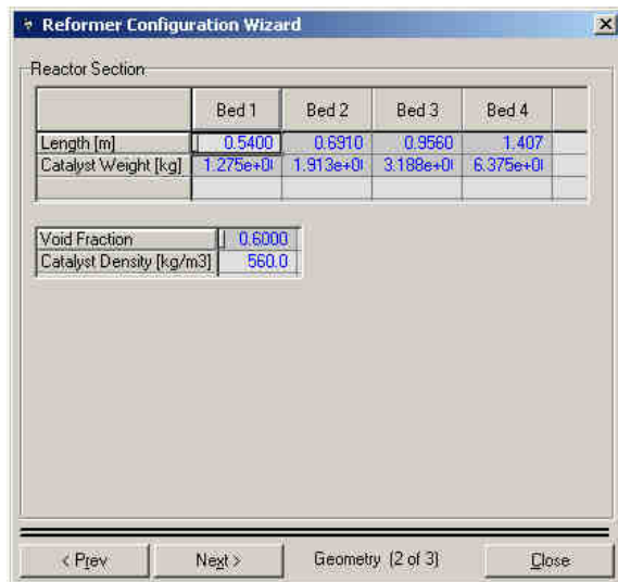
Figure 5.13: Reactor dimensions and Catalyst loadings
