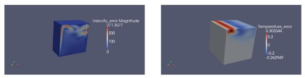
Fig. 9. ROM-G errors profile (left-side: velocity error, right-side: temperature error) - Case two.
