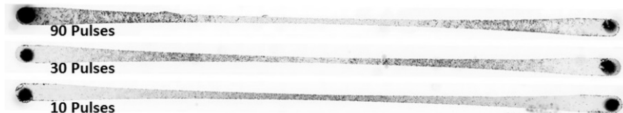
Figure 2-12. Uptake of 4kDa FITC dextran after application of different number of pulses
