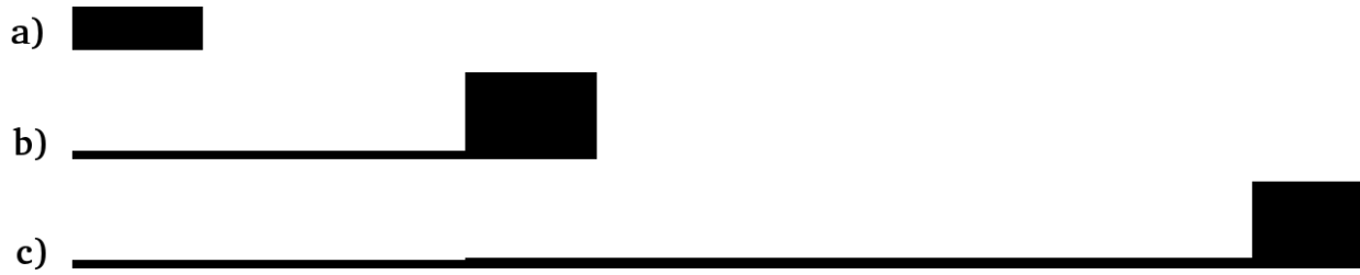
Figure 3.4: Geometries simulated in the electron verification test case: (a) \tilde{L} = 3 cm, (b) \tilde{L} = 12 cm, and (c) \tilde{L} = 29 cm. The geometries shown represent the 2D computational domain with the lower boundary as the axis of symmetry.
