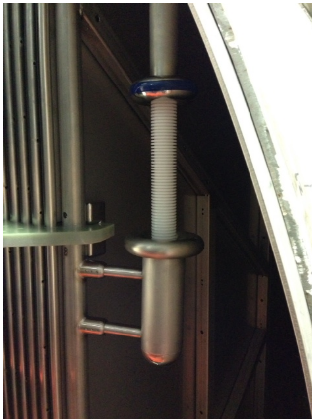
Figure 25. The production HV feedthrough inserted into the cathode receptacle cup inside the cryostat.
