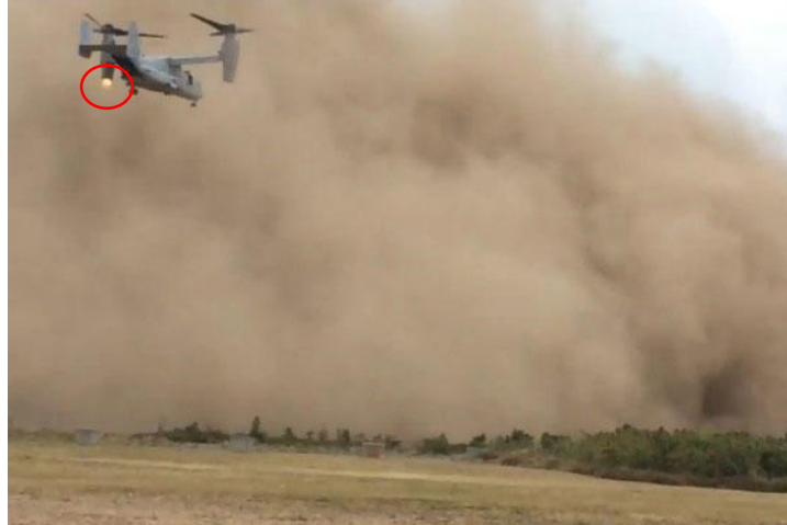
Figure 2: An Osprey V-22 experiencing an engine flameout (highlighted by the circle) before crashing during a training exercise in Bellows, Hawaii [21].
