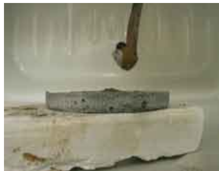
Figure 4. Regolith glass on tip of thermocouple
