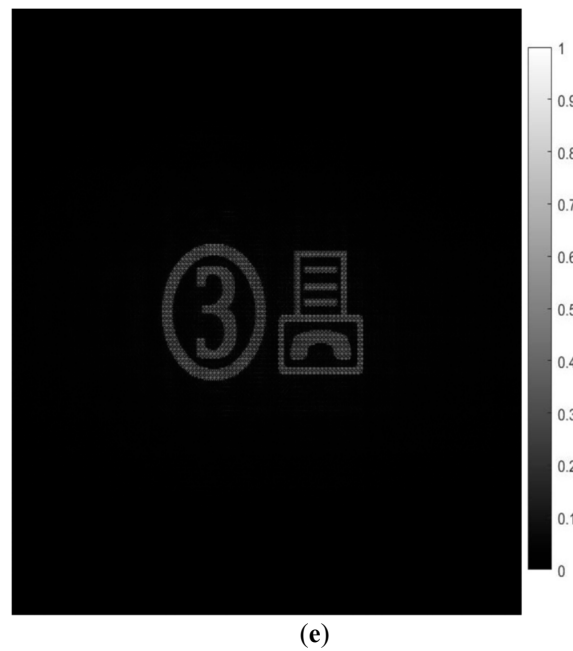
Figure 2. (a) Source image, (b) reconstructed image with the phase component of the hologram of the source image, mostly invisible with most of the contents removed but with slight edge information, (c–e) reconstructed images of the sampled phase-only hologram (SPOH) of the source image with down-sampling factor \tau = 8, 12, and 16, respectively.
