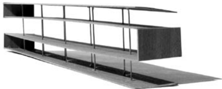
final system for supporting structure
