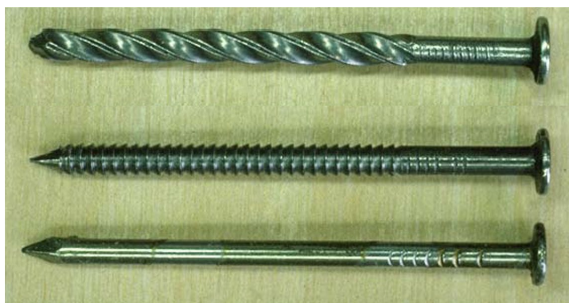
Figure 1. Common nail types used for pallet construction: (top to bottom) helically threaded nails, annularly threaded nails, and plain-shank nails.
