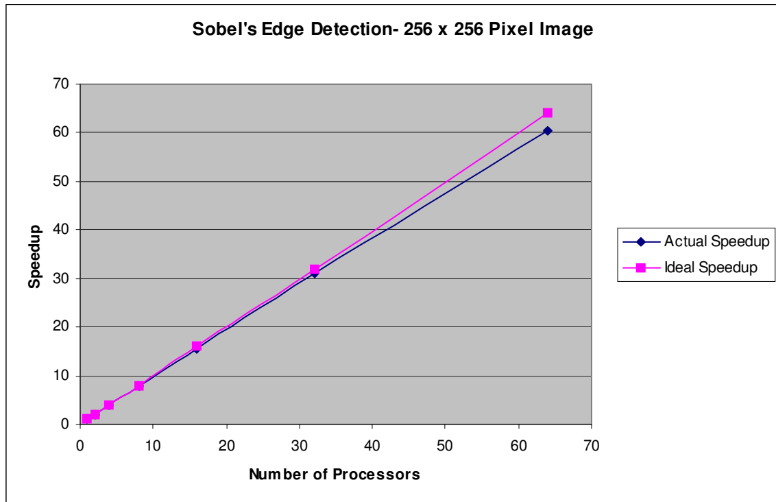
Figure 6.5: Sobel's Edge detection Speedup
