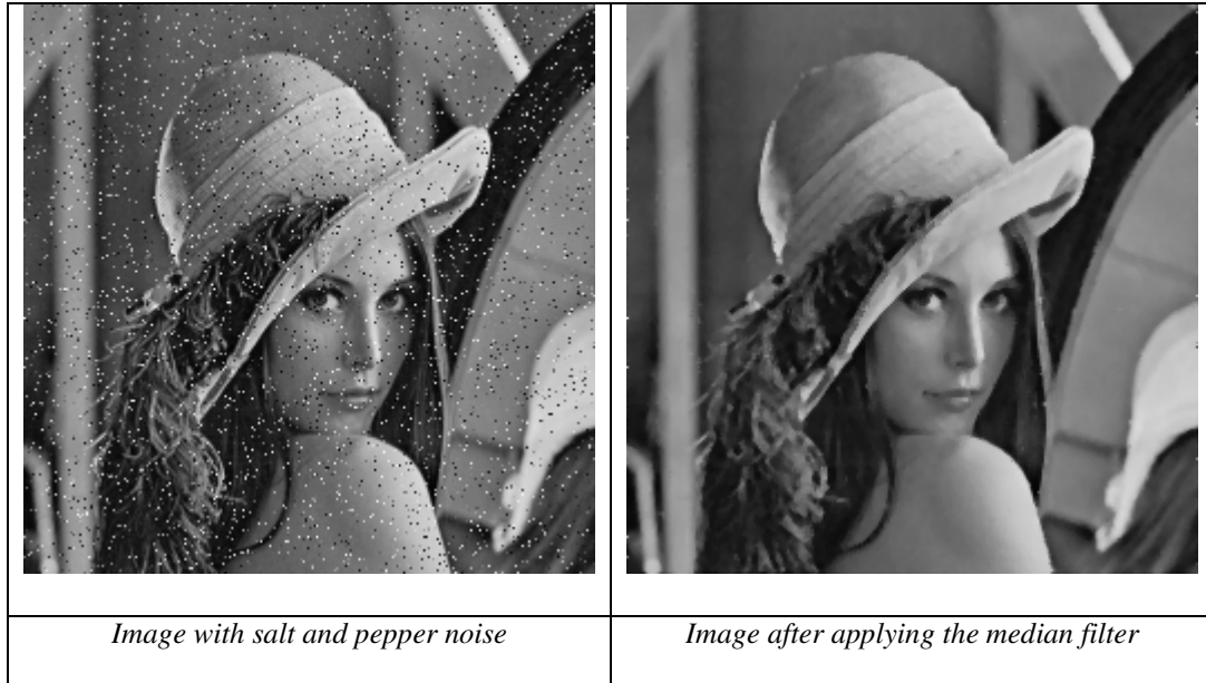
Figure 5.10: Image with noise and image after applying the median filter
