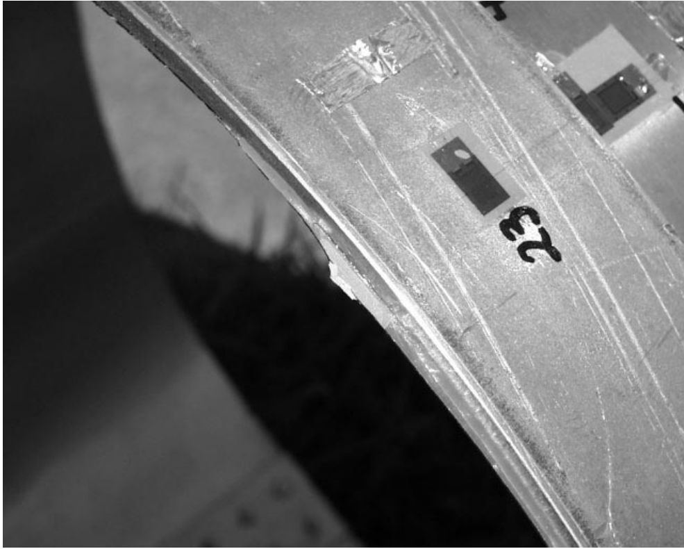
Fig. 2.5 A Photograph of the surface of the failed specimen showing crack bifurcation, turns, and the circumferential paths.
