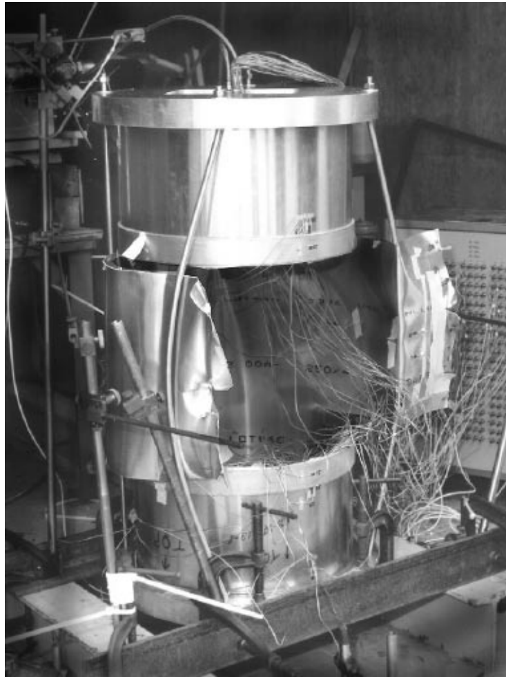
Fig. 2.4 Photograph of the failed stiffened cylindrical shell.
