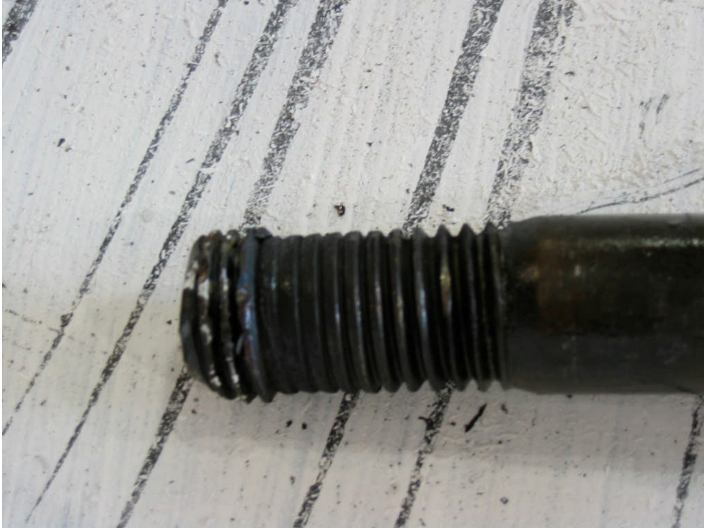
FIGURE 4.34: MRE1/3-1.25-1.5-72 TYPICAL BOLT WITH STRIPPED THREADS
