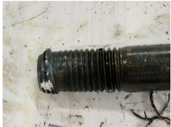
Close-Up of Stripped Threads of Bolt from Far Flange
