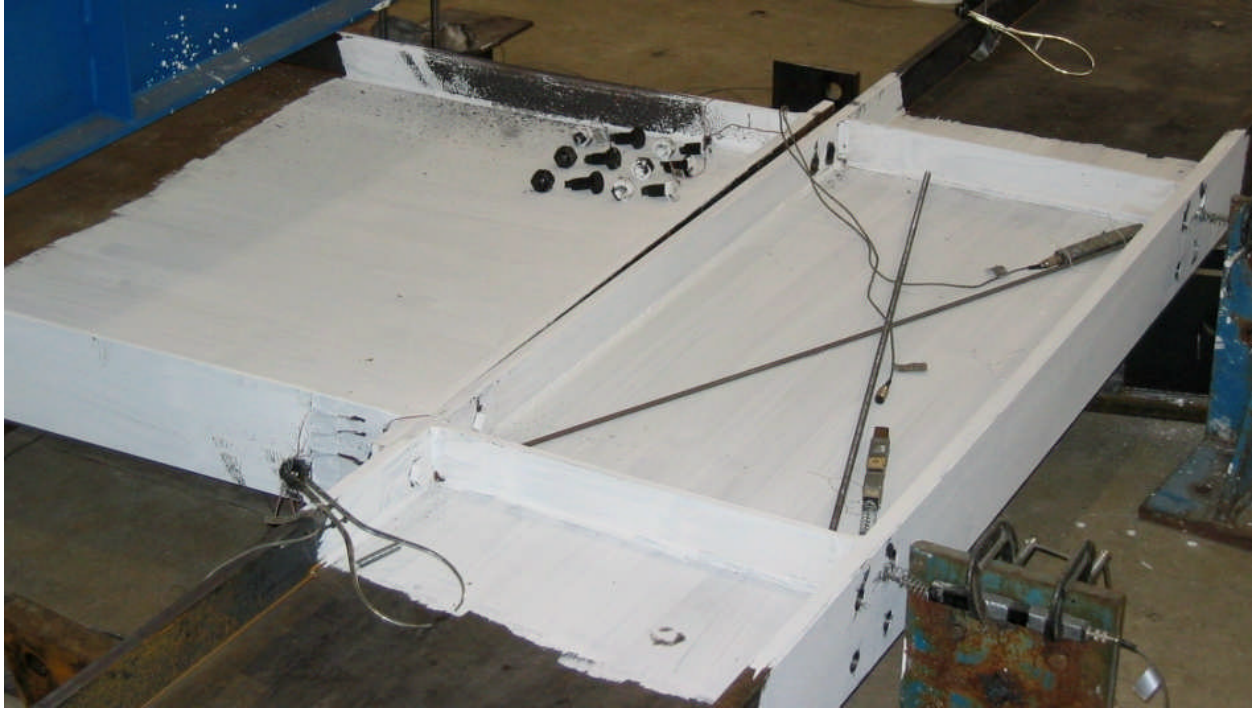
FIGURE 4.23: MRE1/2-1.0-1.0-60 B AFTER BOLT RUPTURE
