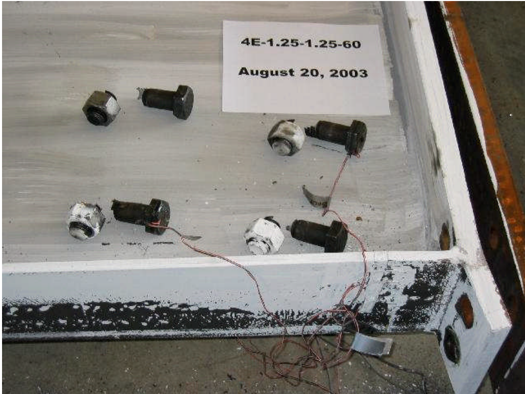
FIGURE 4.14: 4E-1.25-1.25-60 A AFTER BOLT RUPTURE
