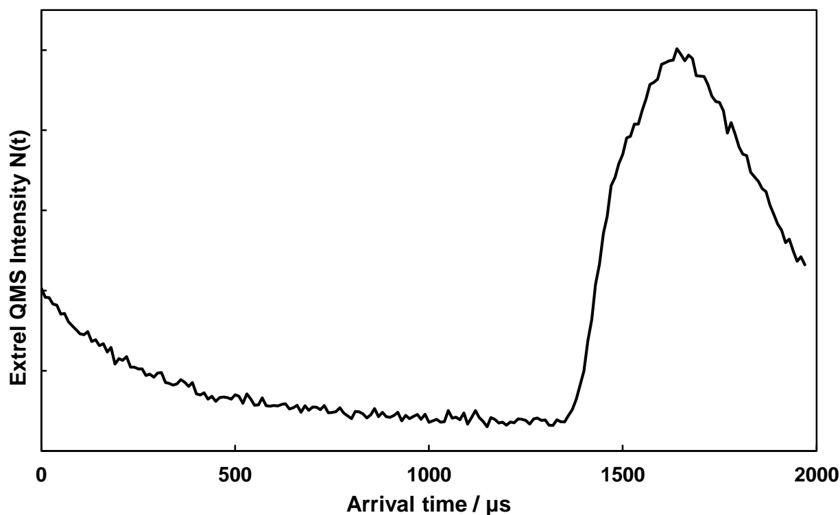
Figure 3.8 The original TOF distribution (raw data, as recorded) of C 2 H 2 in the C 2 H 2 /H 2 beam after colliding with a CH 3 -SAM.
