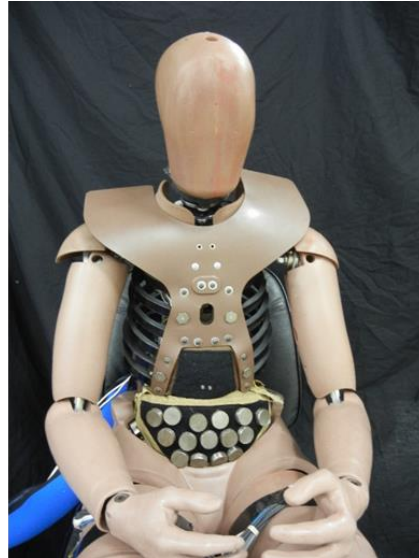
Figure 5.1: Schematic of the APTS abdomen (left) and THOR-M instrumented with the APTS (right).
