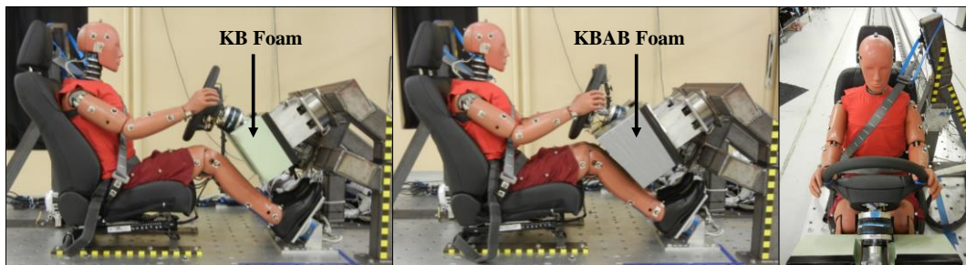
Figure 2.2: Sled test setup side view for KB condition (left), side view for KBAB condition (middle), and front view (right).
