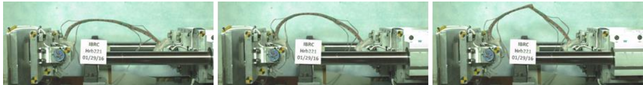
Figure 8.4: Video stills from a bending test with the rib in the initial position (left), displaced before fracture (middle), and during fracture (right).
