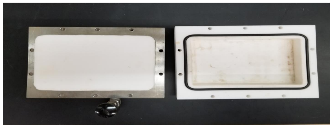
Figure D. 15. The fabricated Teflon hydrolysis chamber.
