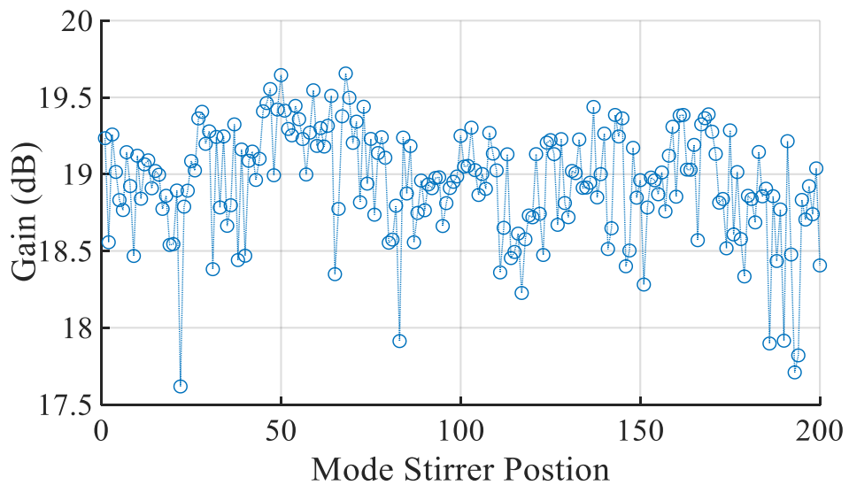
Figure 3-11. Compression Gain over 200 different stirrer positions. Mode stirrer is automatically controlled using MATLAB and a stepper motor such that the entire pulse compression process is accomplished through automated equipment control. Gain is seen to vary from 17.6 dB to 19.7 dB with a mean of 18.9 dB. Inset shows single-paddle mode stirrer attached to shaft below lid.
