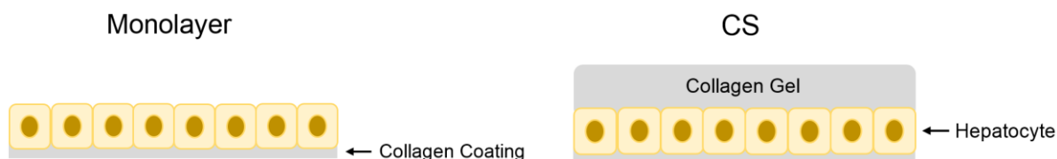
Figure 2.1: Schematic representing iPSC-Heps in monolayer and CS culture models. The iPSC-Heps are maintained as a confluent layer seeded onto a collagen coating in the monolayer model. CS model has a 1.1 mg/ml collagen gel added onto the confluent layer of cells.
