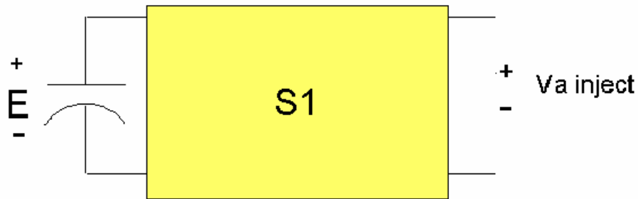
Figure 3.8 - Switching Model of the H-Bridge Converter.
