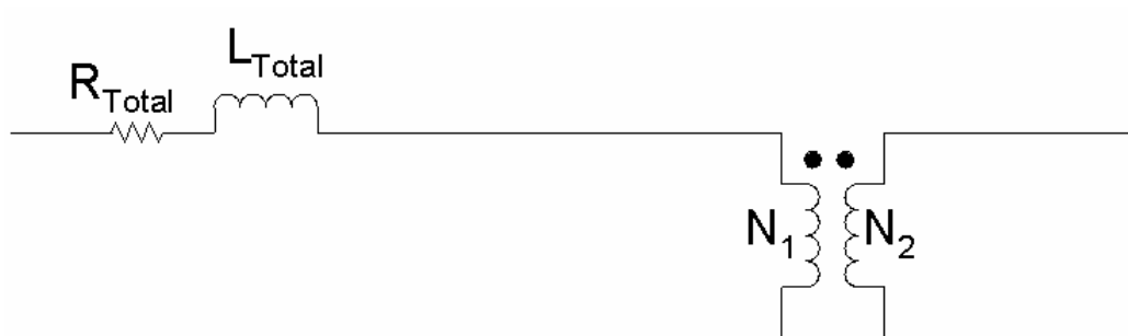
Figure 3.14 - Simplified Transformer Equivalent Circuit.
