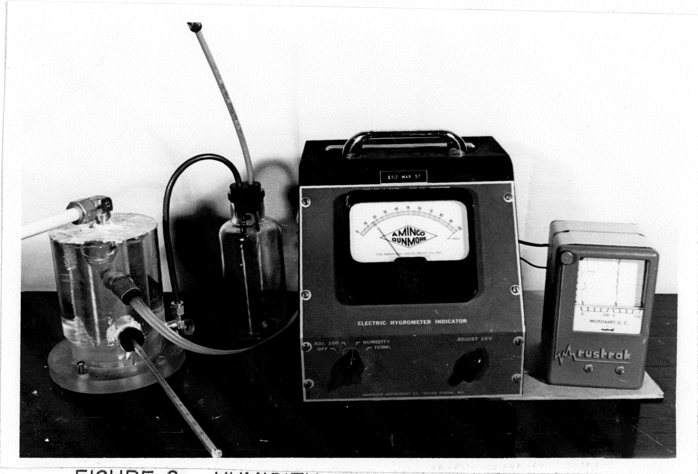
FIGURE 6. HUMIDITY MONITORING EQUIPMENT
