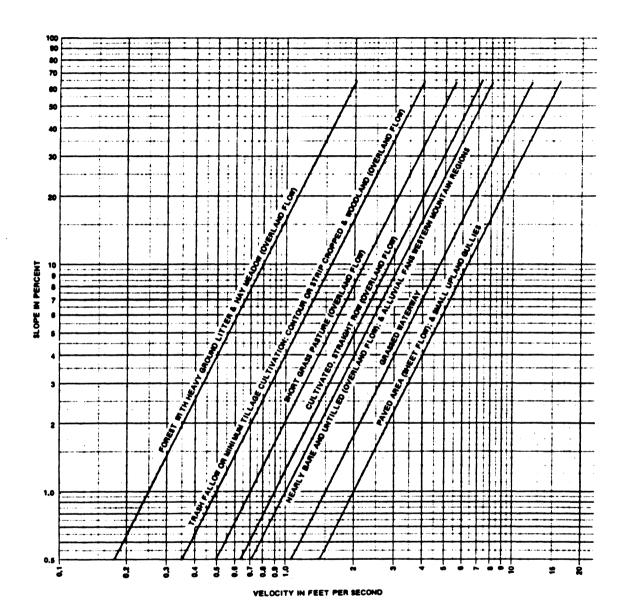
Figure 3. SCS Overland Flow Velocities (SCS TR - 55, 1975)
