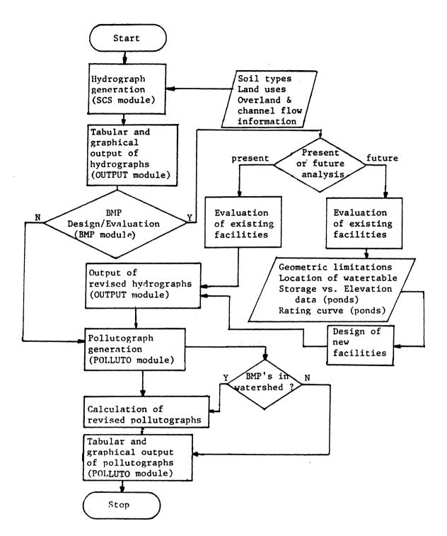
Figure 9. Flow Chart for Software Package "BMPSOFT"
