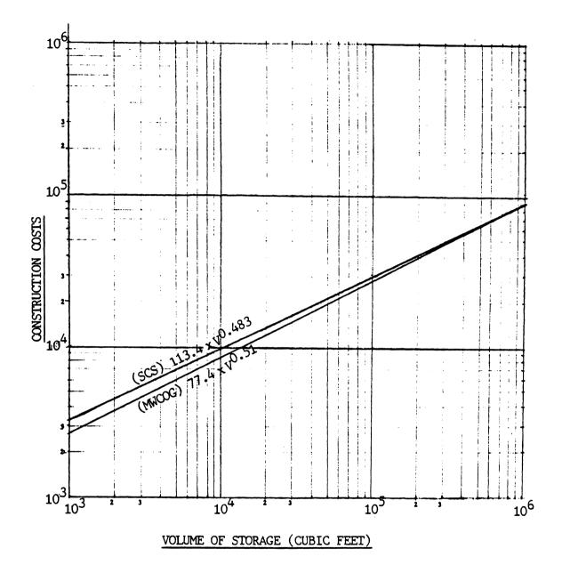
Figure 8. Relationship Between Detention Pond Construction Cost and Storage Volume (MWCOG 12-82)
