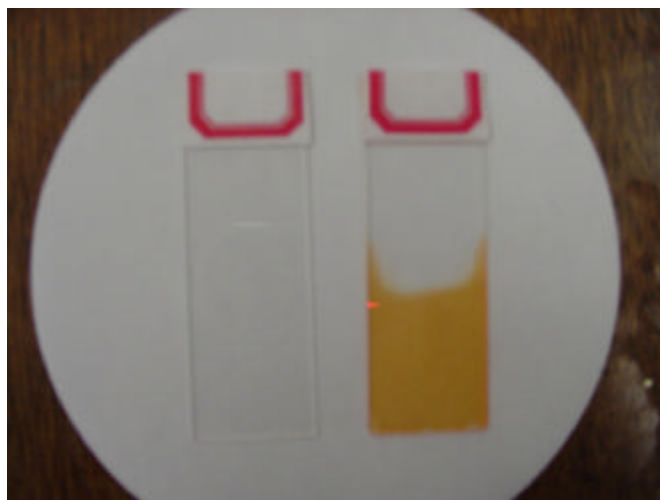
Figure 3.4 Two typical ESA films. Left: PDDA/PSS. Right: PDDA/PS-119.
