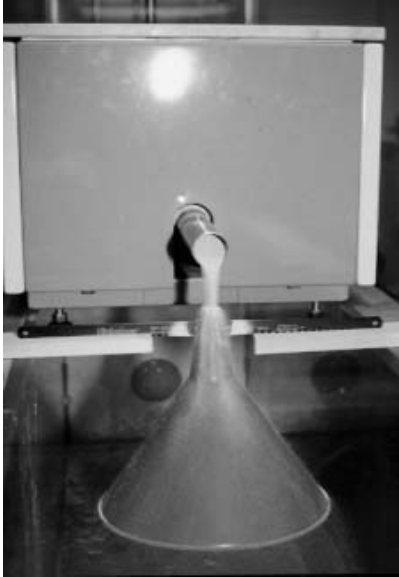
Figure 2.3 - Sediment Auger Mounted on Top of Flume
