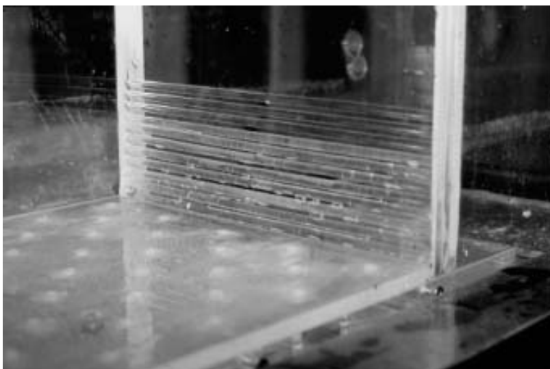
Figure 2.2 - Stoplogs Used to Establish Uniform Flow
