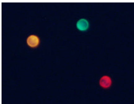
Figure 4. CdSe quantum dots embedded in polystyrene microspheres emitting at three distinct visible wavelengths simultaneously, all under the same ultraviolet light source.
