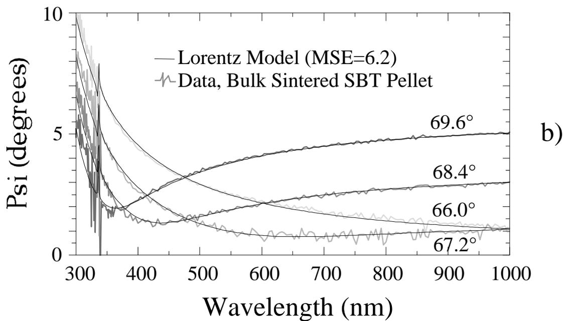
Figure 1-2. VASE spectra from a bulk polycrystalline SBT sample with 2% voids. Delta and psi spectra were fit by a Lorentz dispersion model with absorption at  $5.25 \pm 0.2$  eV and  $3.688 \pm 0.002$  eV, yielding the bulk dispersion curve in Figure 1.
