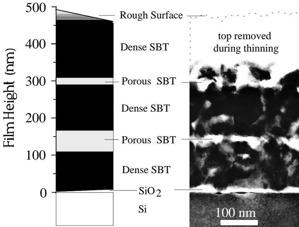
Figure 1-6. SBT/Si film with 3 MOD layers. a) Model C followed the shape of the observed delta spectrum much better than a 1-layer model. b) Model C included porosity between MOD layers, and graded transitions at the top and bottom surfaces. c) Cross-sectional TEM confirmed the thickness estimates of dense and porous layers made by VASE in model C. Considering that VASE optically characterized a region 1000 times larger than the area shown by TEM, the profiles showed remarkable agreement.
