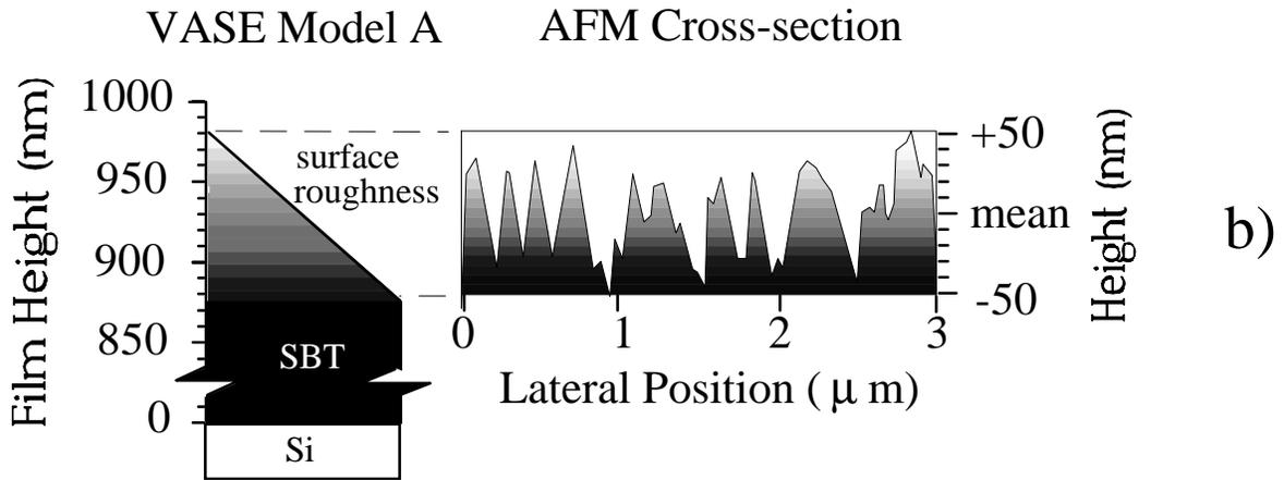
Figure 1-3. SBT/Si film made by PLD. a) Model A fit the VASE spectrum better than a 1-layer model. b) Including a linear transition from SBT to voids, model A accurately predicted the depth of surface roughness, as shown in the AFM cross-section.
