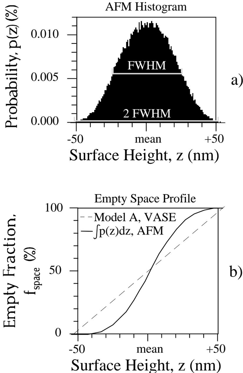
Figure 1-4. Comparison of surface empty space profiles from AFM and VASE.
