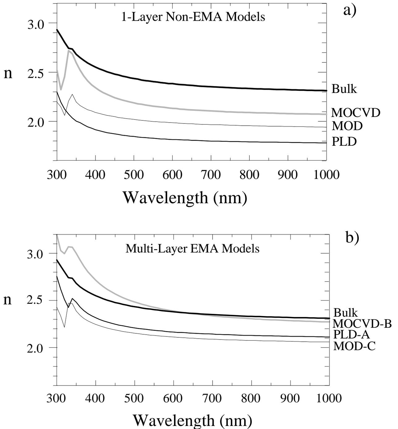
Figure 1-1. Comparing SBT refractive index,  $n$ , curves from bulk samples and thin films (MOCVD, MOD, & PLD). a) 1-layer VASE models underestimated  $n$  in thin films. b) By simulating observed void profiles with EMA layers, models A, B, and C obtained SBT optical properties from thin films that were closer to bulk values.
