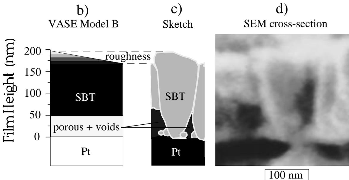
Figure 1-5. SBT/Pt film made by MOCVD. a) The  $\Delta$  spectrum of this dense film was reasonably modeled as a single layer. b) Model B improved the fit by including surface roughness and voids near the base of the film. c) A sketch illustrates how voids could remain near the Pt substrate between kernal-shaped grains. d) Features seen in a SEM cross-section (dark holes between SBT grains, shallow surface roughness, and overall film thickness) were consistent with VASE model B.
