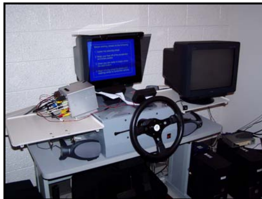
Figure 3.7 External Computer, Steering Wheel, and LCD's
